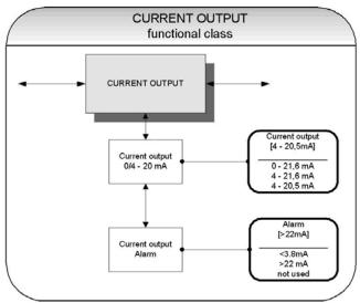
The current output is generally assigned to volume flow.
