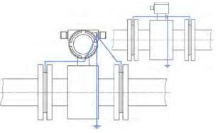
Protection washers or protection rings can also be used as earthing component; or special earthing electrodes, incorporated in the sensor, may be installed.
