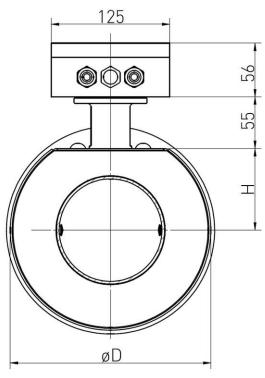
The dimensions L, W, D and H correspond to the values of the table on the compact device ( $\rightarrow$  § 11.3.1).
