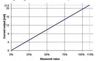
The standard range from 4 to 21.6 mA uses the measuring range up to 110 %.
