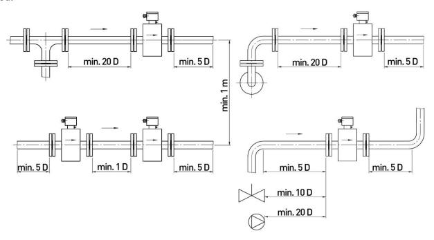
If several sensors are installed in series, the distance between each sensor must be equal to the length of one sensor. If two or more sensors are to be installed in parallel, the distance between sensors must be at least 1 m.
