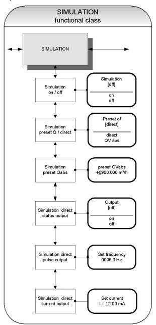
If simulation mode is activated, all output signals will be generated depending on the selected items. This function enables testing of peripherals connected to the device without water flow.
