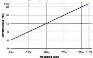
The range from 4 to 20,5 mA is according to the NAMUR-recommendation and uses the measuring range up 104%.
