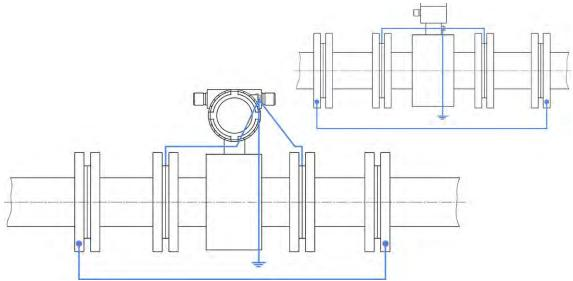
An electrical connection occurring between the sensor and any material used for the installation must be avoided. Insulating segments must be installed between the sensor and the pipeline (e.g. PVC pipes or similar).
